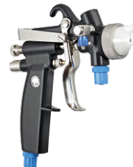
Standard spray gun PILOT III-2K : PTFE-coated gun body for applying 2C adhesives
